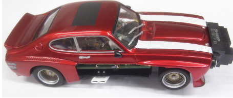
Fig. 2. Carrera Ford Capri RS Tuner 3 with a hole cut in the side revealing the controller PCB inside. IR proximity sensor attached to the front.
