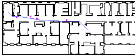
Figure 5.14: Example path of Basic Theta* in hospital environment with all four new obstacles
