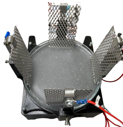
Figure 2.3: Shot of the electrode array with the electrodes submerged in the fluid. Fluid is also seeded with particles for measurement of the velocity field.
