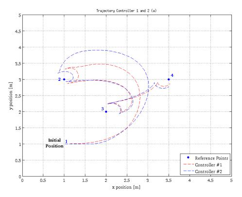
Figure 4.30: Trajectories comparison, from initial condition to point 4
