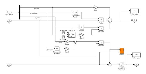
Figure 4.16: Controller Implemented in Simulink
