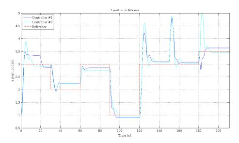
Figure 4.25: Y Position vs Reference Results and Comparison
