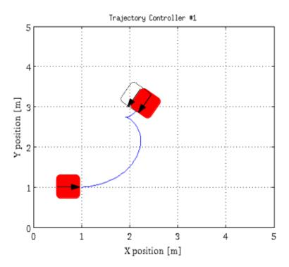
FIGURE 4.15: Trajectory followed and final position for Controller Kanayama
