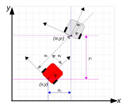
FIGURE 4.4: Error Geometry from Current to Reference Position
