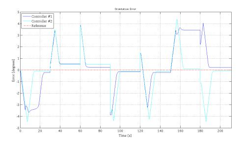
Figure 4.29: Orientation Error Comparison
