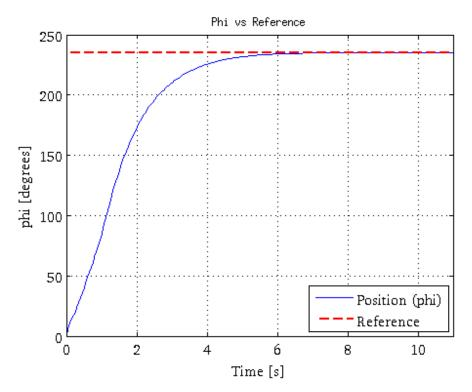
Figure 4.11:  $\phi$  Position vs Reference Results – Kanayama
