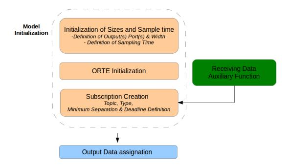
FIGURE 3.2: Subscriber S-Function Diagram
