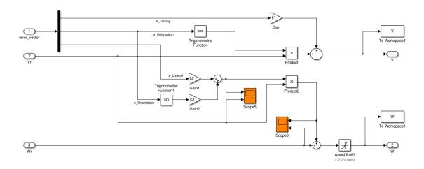
FIGURE 4.5: Controller Kanayama Implemented in Simulink
