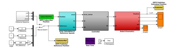
FIGURE 4.8: Simulink Final Implementation
