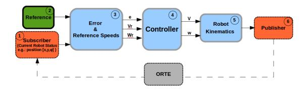
FIGURE 4.1: High Level Control Diagram
