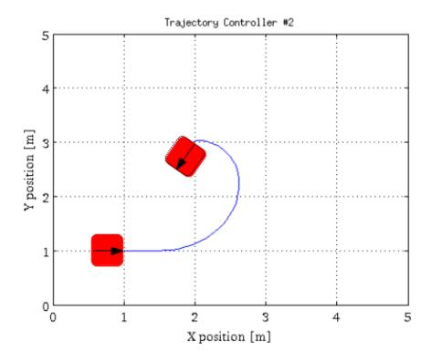
FIGURE 4.23: Trajectory followed and final position for Controller Sanhoury
