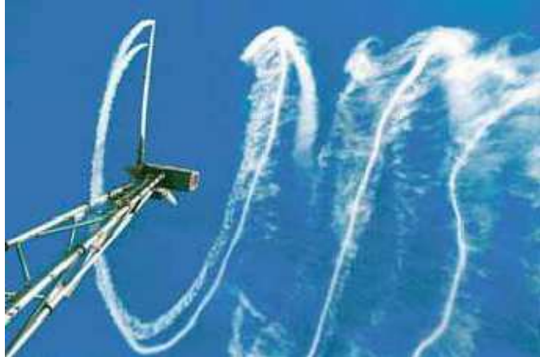
Figure 2-12: An experiment which demonstrates the rotational behavior of the wind passing through the turbine (wake) and also the change of the volume of air leaving the turbine (smoke spreads away from the turbine). 15
