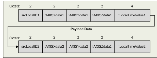
Figure 6.3: TOS message Payload Data field structure.
