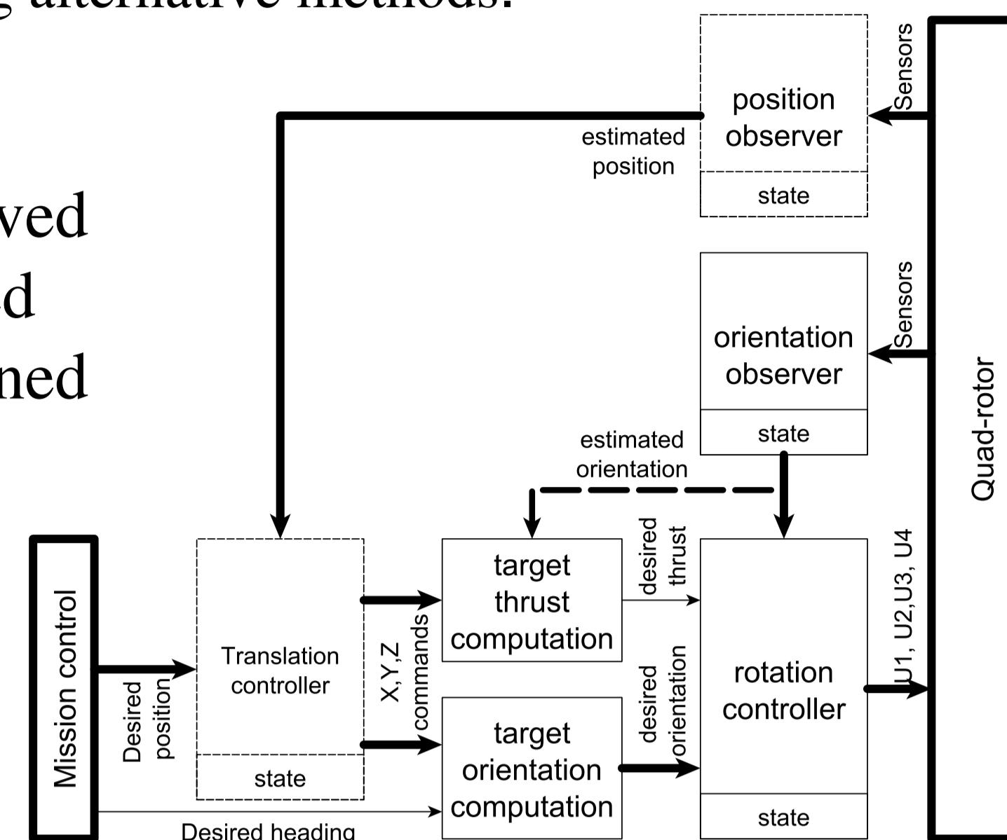
Euler angles have been sucessfully used for control of fixed-wing aircraft as natural representation of errors from straightforward flight. Nevertheless, for an omnidirectional aircraft, non-linearities arise when moving far from the zero orientation state. **Quaternions offer a significant advantage in terms of mathematical robustness and not suffering from singularities.**
