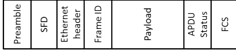
Figure 1: Profinet IRT message
