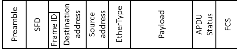
Figure 2: Profinet IRT message for fast forwarding
