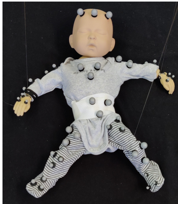
Figure 4.7: The layout of marker clusters secured to the doll individually using tape. The different sizes of the markers were irrelevant for this experiment.
