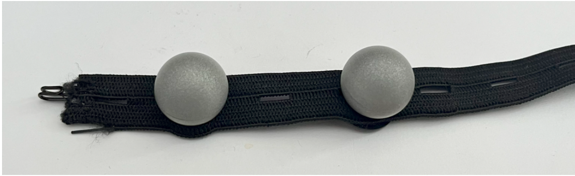
Figure 4.4: An elastic band with buttonholes with two markers secured and a hook for attachment.
