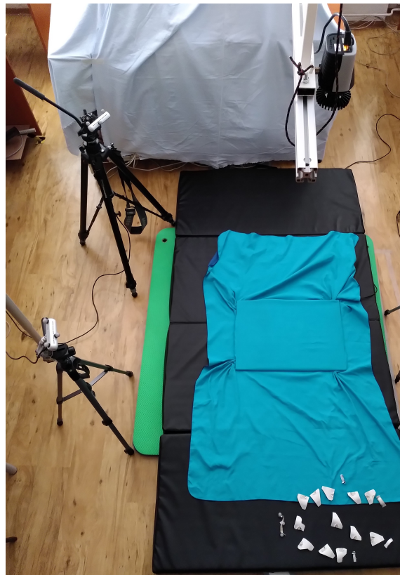
Figure 4.13: The setup for the infant recording consisted of two Intel RealSense D455 RGB-D cameras on tripods, an RGB Qualisys Miquis video camera mounted on a rig above the infant and eight infrared cameras (not visible in this figure). The infant was positioned on a washable towel on multiple mats. In the bottom of the figure, there are prepared markers layed out in the formation they will be put on the infant.
