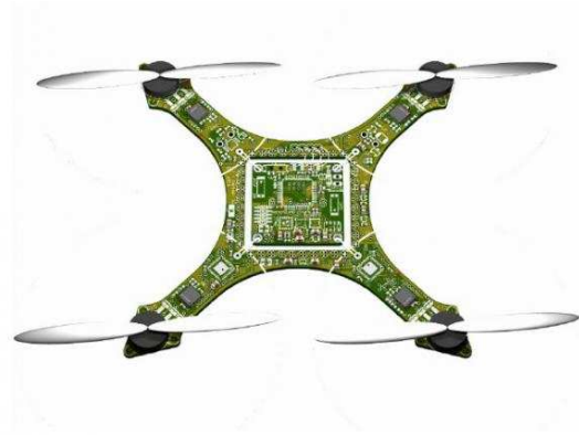
Figure 1.2: NANOQUAD. Prototype of NanoQUad (a very small quadcopter) developed at AA4CC by Jaromír Dvořák. Copyright(c) 2012 by AA4CC.
