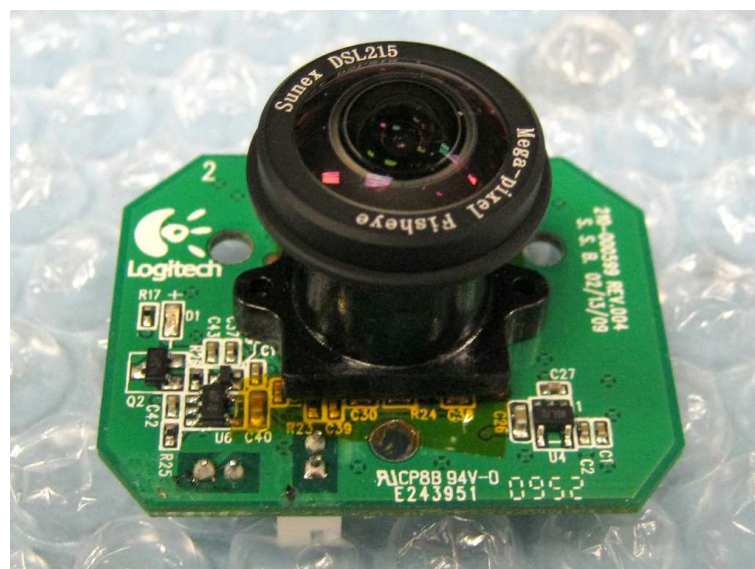
Figure B.4: Logitech Webcam C600 with mounted and sealed DSL125
