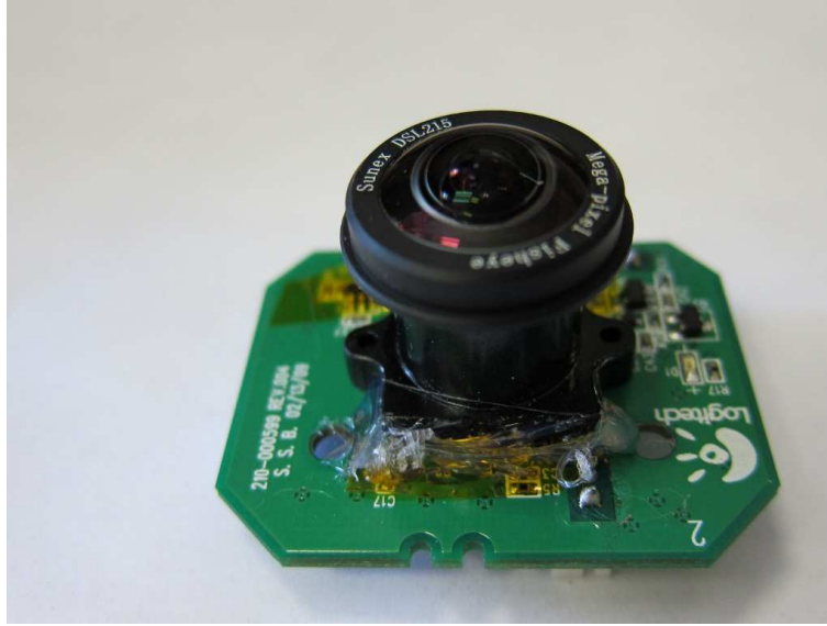
Figure 4.15: Logitech Webcam C600 with DSL125 lens without a cover box
