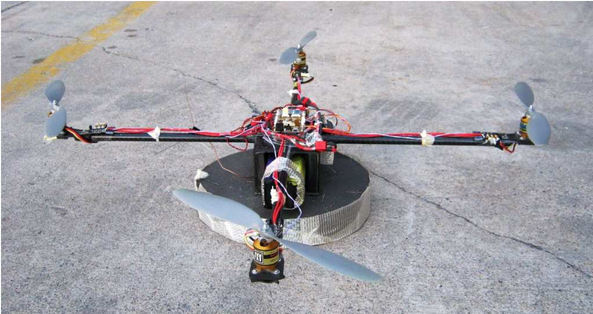
Figure A.1: AggieVTOL without landing gear (Styrofoam landing pad is used instead during attitude controllers tuning)
