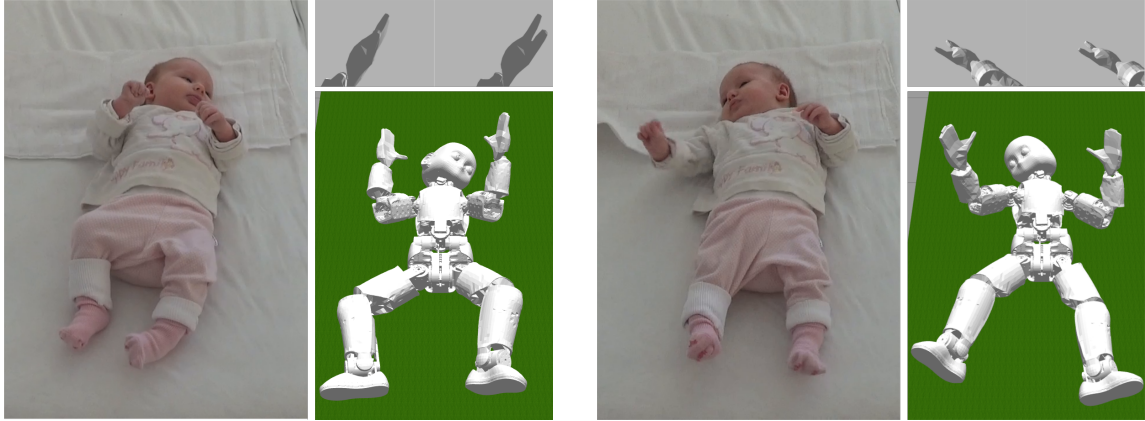
Figure 5.4: Transferred motion from baby to iCub with vision output.
