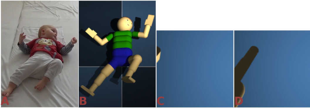
Figure 5.6: Transferred motion from baby to MIMo with a visual output. (A) real infant, (B) MIMo, (C) right eye, (D) left eye.
