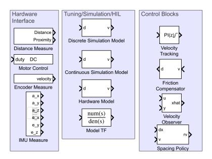
Figure 2.2: Schematic of the library with common slotcar blocks
