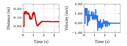
Figure 3.9: Testing ACC controller when driving into a wall at maximum speed
