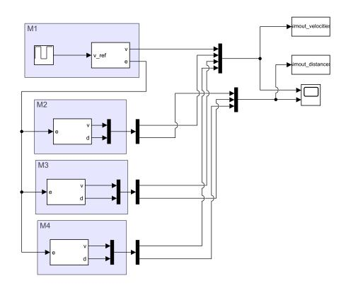
Figure A.1: Simulink block diagram of drive4CACC
