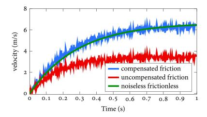
Figure 3.8: Simulated comparison of step response of slotcar models with friction and Gaussian measurement noise to the linear transfer function
