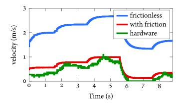
Figure 3.2: Comparison of hardware in the loop measurement and models with and without friction
