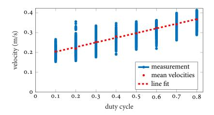
Figure 3.3: Measured controller effort (duty cycle) for different reference velocities with mean values fitted by a line
