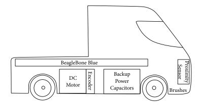
Figure 1.1: Layout of slotcar hardware from the side
