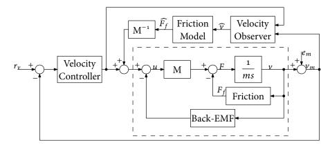
Figure 3.7: Block diagram of friction compensation
