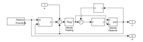
Figure A.4: Inner scheme implementing the CACC controller
