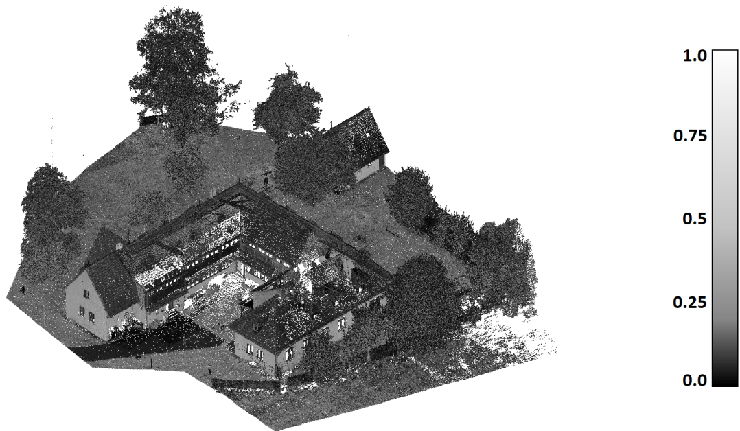
Figure 6.9: Reference 3D point cloud from Leica BLK360 laser scanner
