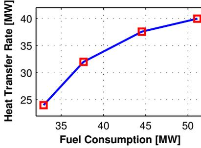
**Figure 3.3:** Fuel consumption characteristics of the boiler B1
