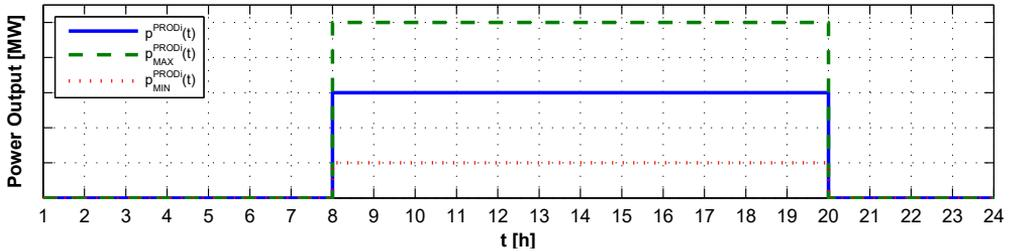
**Figure 1.4:** Definition of a generic daily peak load product (an example of a feasible value of contracted volume in blue)
