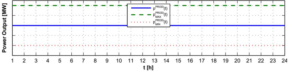
**Figure 1.3:** Definition of a generic daily base load product (an example of a feasible value of contracted volume in blue)
