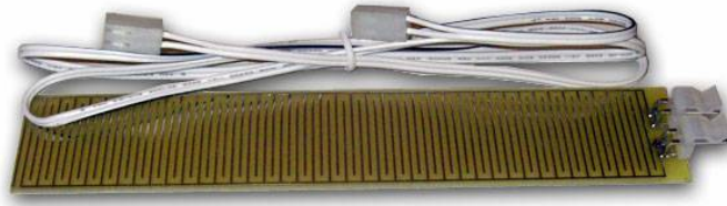
Figure 2.5: Water leak sensor
