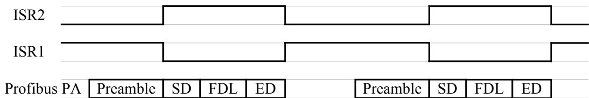
Figure 5-5: Waveform of Interrupt Service Routines
