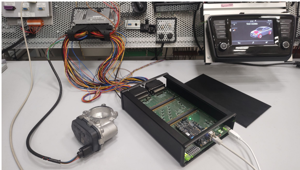
Figure 1.1: The photo of the developed simulator connected to the ECU and the Škoda breadboard. The simulator enclosure is disassembled to show the 50-pin D-Sub connectors.
