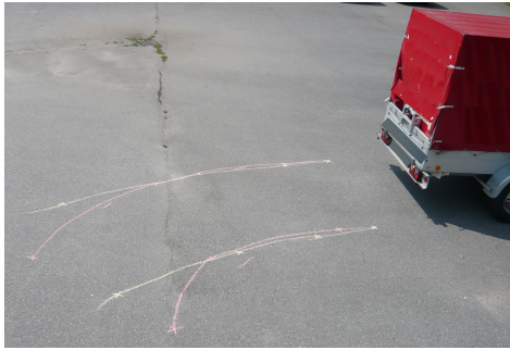
Figure 8.5: Used method of performance test for the single-axle trailer
