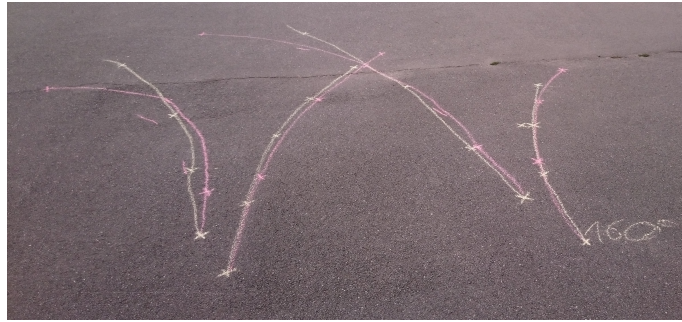
Figure 8.6: Comparison of the driving path for two different steering angles for a single-axle trailer
