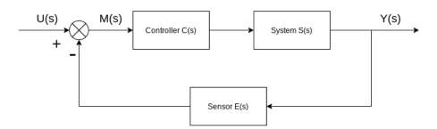
Figure 2.1: Feedback loop with descriptions
