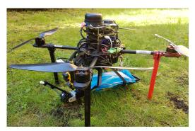
(a) UAV with mounted fire extinguisher
