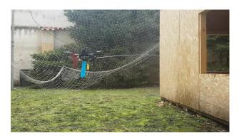
Figure 5.1: Pump (Comet) and nozzle test on the drone without manipulator and bag holder
