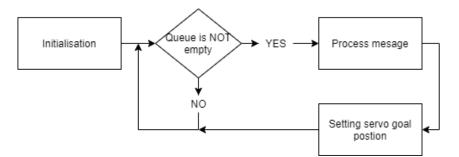
Figure 4.3: Program on microcontroller
