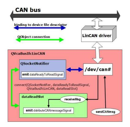
Figure 7.2: CAN bus monitoring using the local connection to LinCAN driver
