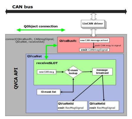
Figure 7.4: QVCA architecture and message distribution
