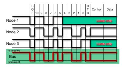
Figure 2.3: CAN data transmition
