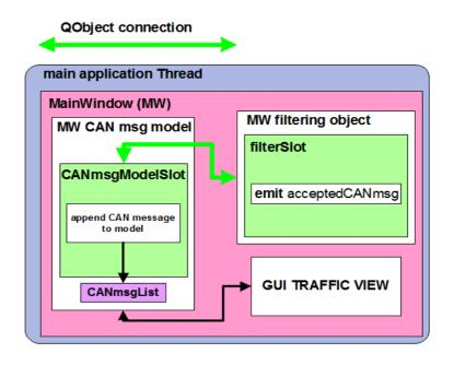
Figure 8.3: QCANalyzer CAN message flow
