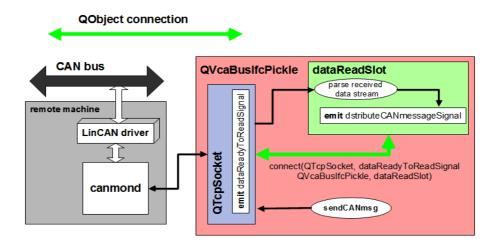
Figure 7.3: CAN bus monitoring using remote connection to LinCAN driver
