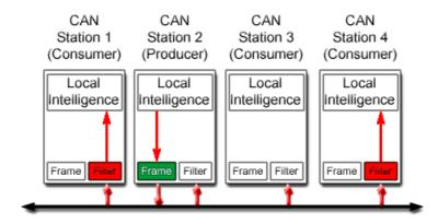
Figure 2.1: CAN Acceptance Filtering
