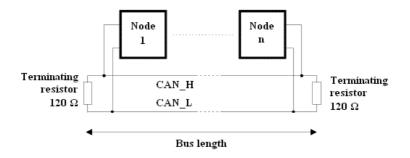
Figure 2.2: CAN network structure according to ISO-11898
