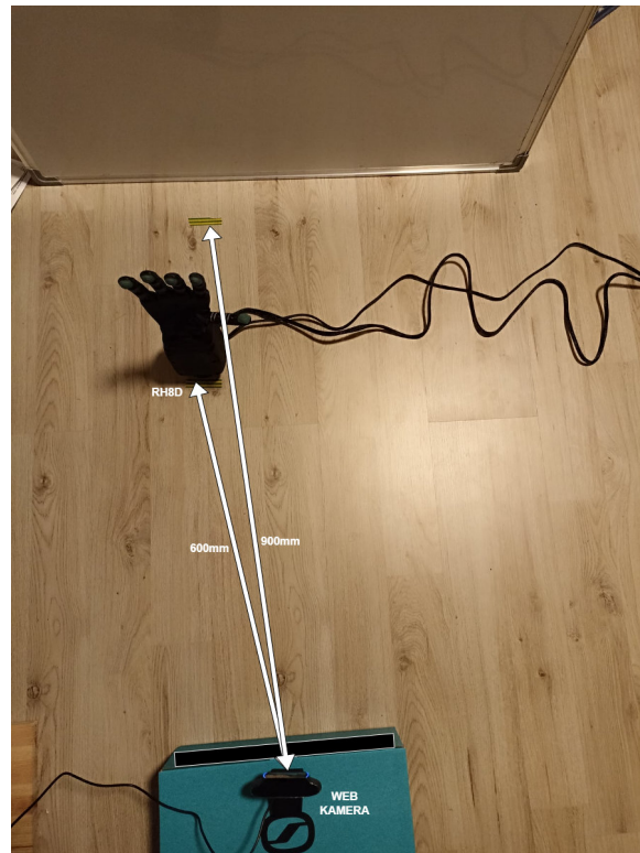
Figure 5.2: RH8D gesture recognition test environment at varied distances and glove usage.
