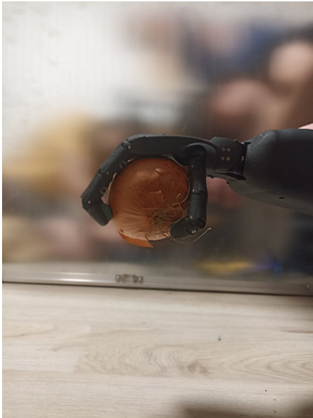
(a) The RH8D robotic hand demonstrates the grasp of a spherical object. The depicted robotic hand holds the onion firmly, showcasing its ability to handle round and smooth surfaces.
