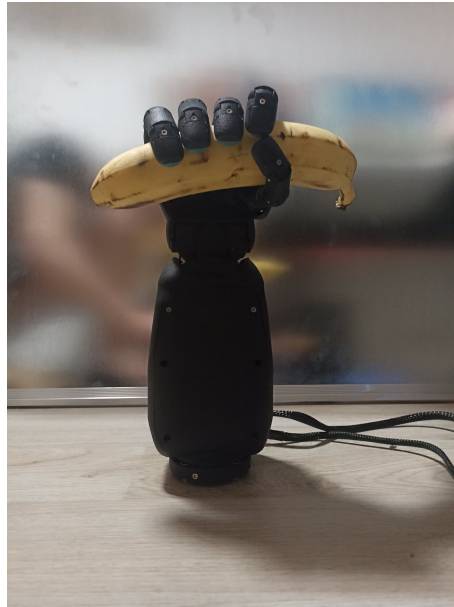
(b) The RH8D robotic hand demonstrates the grasp of a cylindrical object. The image shows the hand securely holding a banana, illustrating the hand's capability to manipulate elongated items.
