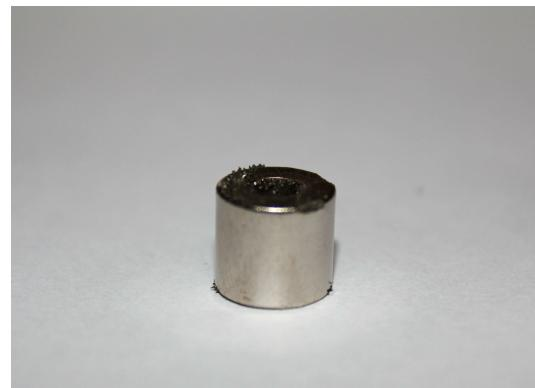
(b) Magnet o velikosti  $d \times v \times a = 9 \text{ mm} \times 10 \text{ mm} \times 4 \text{ mm}$
