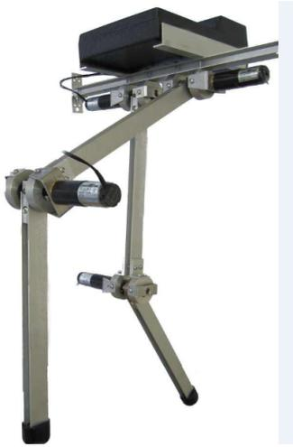
Figure 3.2: Real Acrobot at CVUT.
