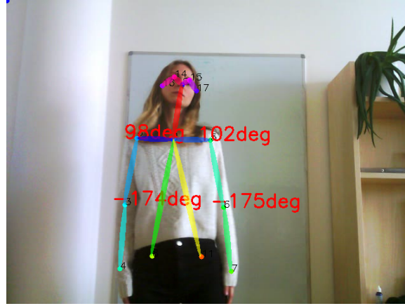
Figure 3.5: Example of the picture from Pepper humanoid robot's camera with the skeleton structure, which was produced by the OpenPose algorithm
