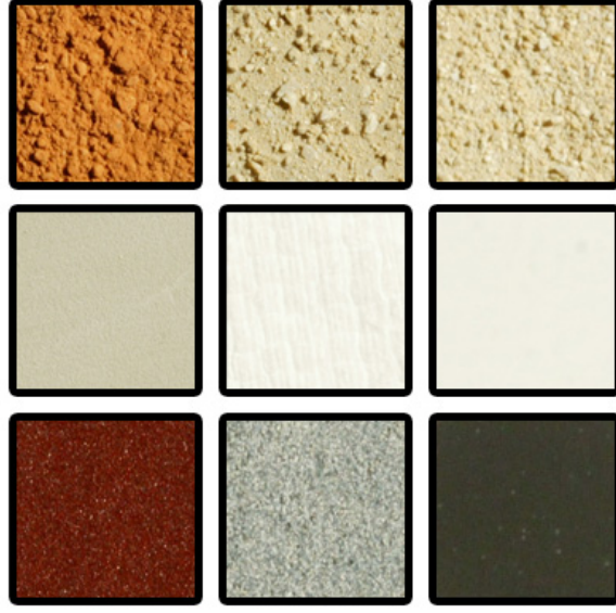
Figure 5.3: Set of investigated real-world material samples. From the top left: red clay, light rough sand, light fine sand, modeller material, cotton pad, white matt painting, abrasive paper, abrasive rock (carborundum), black matt painting.
