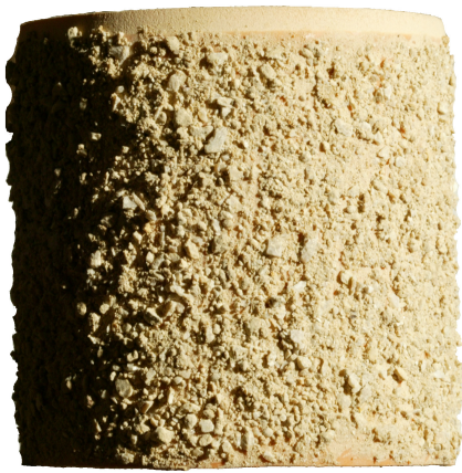
(a) The cylinder model with rough sand on surface. Its size is approximately 10cm in diameter and 10cm in height.
