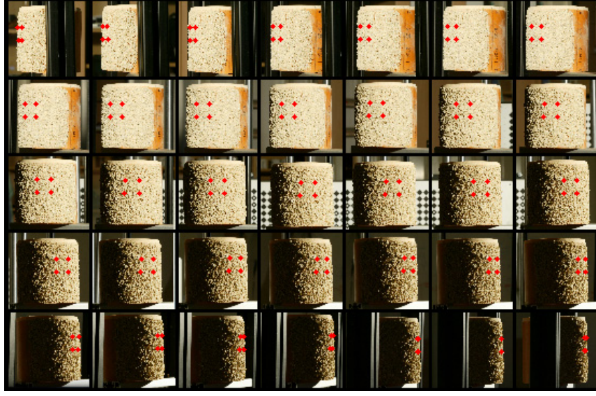
Figure 5.9: Cylinder with projected facet corners. The camera views are -85^\circ in the top left image, increasing when moving right and down to 85^\circ in the bottom right corner.
