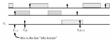
**Note:** We suppose that tasks are in phase (not shown in the figure above) and processor never idles before  $J_{i,k}$  missed its deadline.
