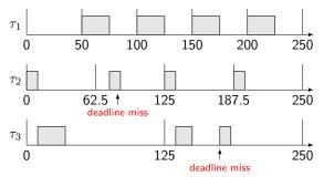
■ DM fails ⇒ RM fails. DM can produce feasible schedule when RM fails.
